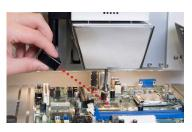
The Closed-Loop, Non-Contact IR Pyrometer monitors and controls the ramp-rate and temperature of the component in real time, by controlling the top and bottom heaters' output throughout the reflow process.
